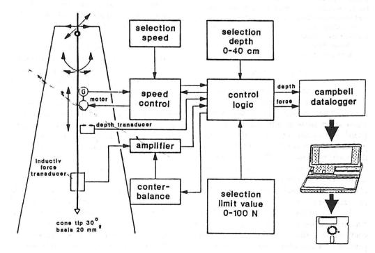
Fig. 1. Experimental setup of penetrometer for the measurement of soil resistance.
